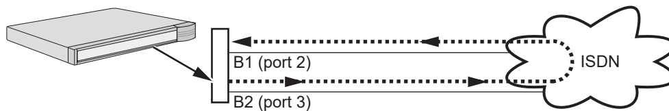
Figure 208: ISDN Loopback Testing
